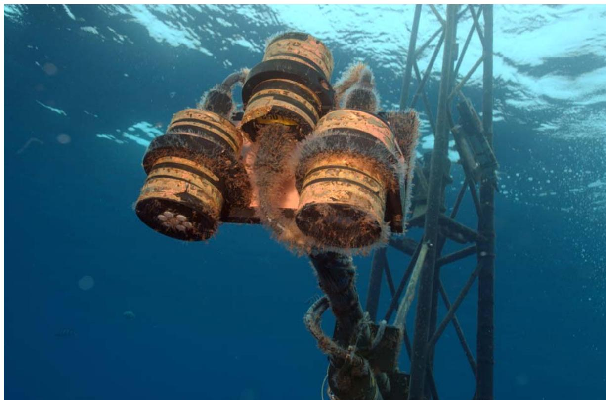
The BOUSSOLE buoy radiometers set measuring *Ed*, *Eu* and *Lu* at 4m depth, colonized by caprellid amphipods (*crustacea*) before cleaning.
